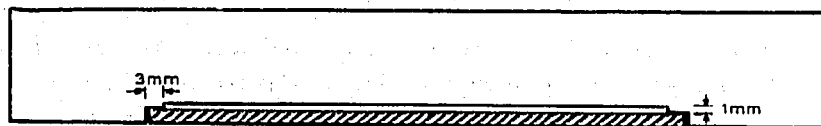
Fig. 1. Plan of the machined brass strip which is 6 mm thick. The hatched area represents the section of the chromatoplate.
